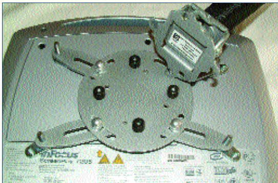
Align the screws of the ceiling mount exactly with the drilled holes at the back of the projector
