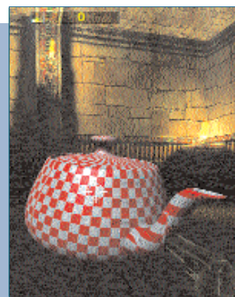
This image shows how bump mapping is used to create the emboss effect on the kettle
